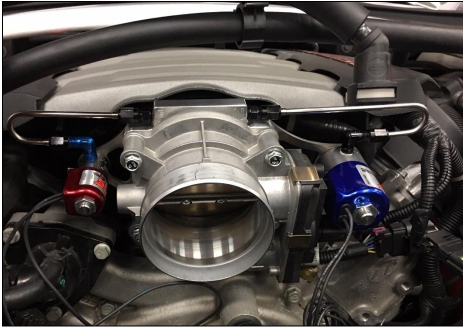
Figure 10 – Hardline Routing and Assembled Plate
