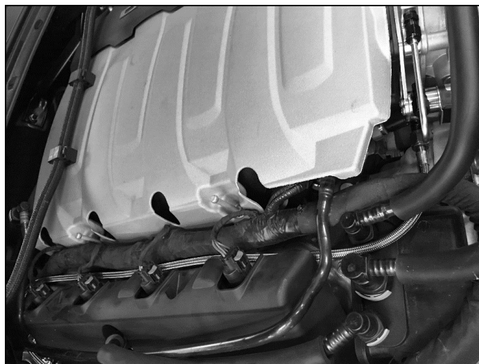
Figure 13 – Fuel Line Routing
