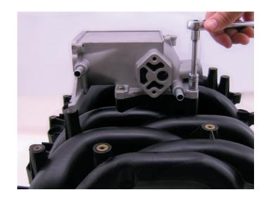
Using the original o-ring or gasket place the nitrous plate on the lower intake manifold. You must be able to read "TOP" on the top of the nitrous plate and the word "FUEL" must be facing to the front of the vehicle
