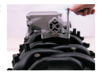
Once the four plate bolts are loosely installed, you may install the provided spacer beneath the support leg of the upper intake manifold and install the final bolt, again do not tighten.
