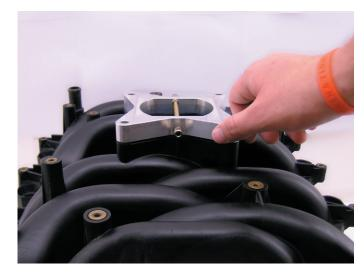
Although no gasket is needed on the underside of the plate, the supplied gasket will be needed between the upper plenum and the nitrous plate.
