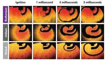
Note: Based on flame kernel growth tests comparing a NGK RUTHENIUM HXTM PSPE® design with Iridium and Nickel J-gap designs.
