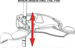
When feeding the pin into the desired slot, take extra care not to puncture the tether, and be sure the pin is aligned with the small hole in the back of the slot. Do not force the pin, it should easily screw in. Watch closely as you insert the pin into the loop to ensure that the pin fits inbetween the tethers, and not outside of them. When tightening the pin, do not overtighten as it will cause damage to the insert. Tighten to 25 in. lbs.
