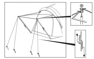
14) Insert the ring on the guide rope around the point and place the awning cap over the guide rope. Stake the other end of the ground with a peg. Adjust length of guide rope.
