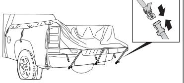
5) Assemble the tent poles by unfolding each section. Below is a list of the poles and the placement.
