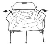
**3)** Locate the tent side straps (3 per side). Loosely attach each strap to the truck's body.
