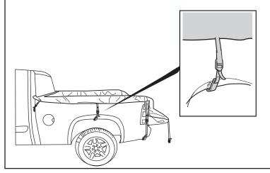
4) Locate the tent tailgate straps (3). Slide the 3 straps with male clip between the truck box and the tailgate. Connect the strap with the male clip to the corrsponding strap with the female clip.
