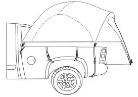
**11)** Attach the rain fly to the tent by clipping the 6 straps (2 per side and 2 at tailgate). Tighten the straps if necessary.
