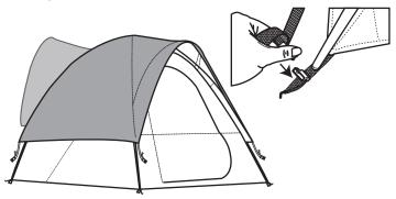
9. A. Slide the pole through the sleeve located above the rainfly door area. Place both ends into the grommet hole at each corner of the rainfly
