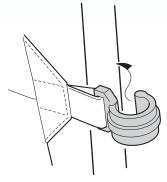
D. Ensure the exhaust pipe is outside the sleeve
