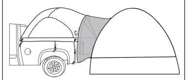
B. Attach the bottom outside J-Hook strap to any part of the wheel well and tighten the strap. Repeat on the opposite side
