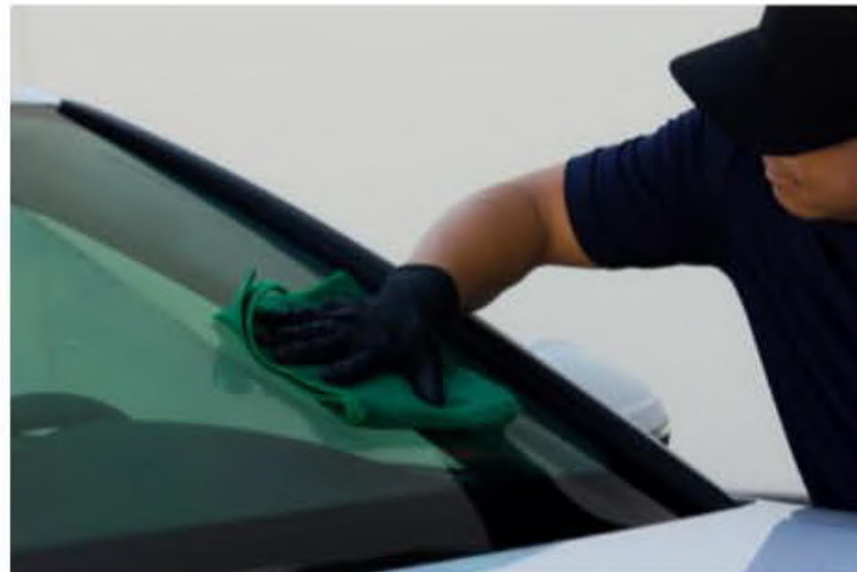
Step 5: Wipe glass surface clean of residual Rain glass sealant
