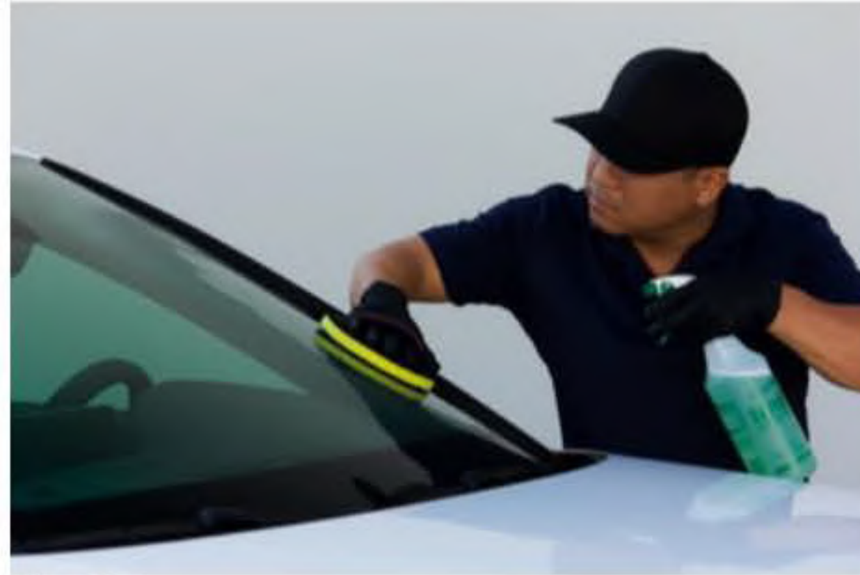
Step 2: With light to medium pressure slide the Autoscrub across the glass surface in a back and forth motion
