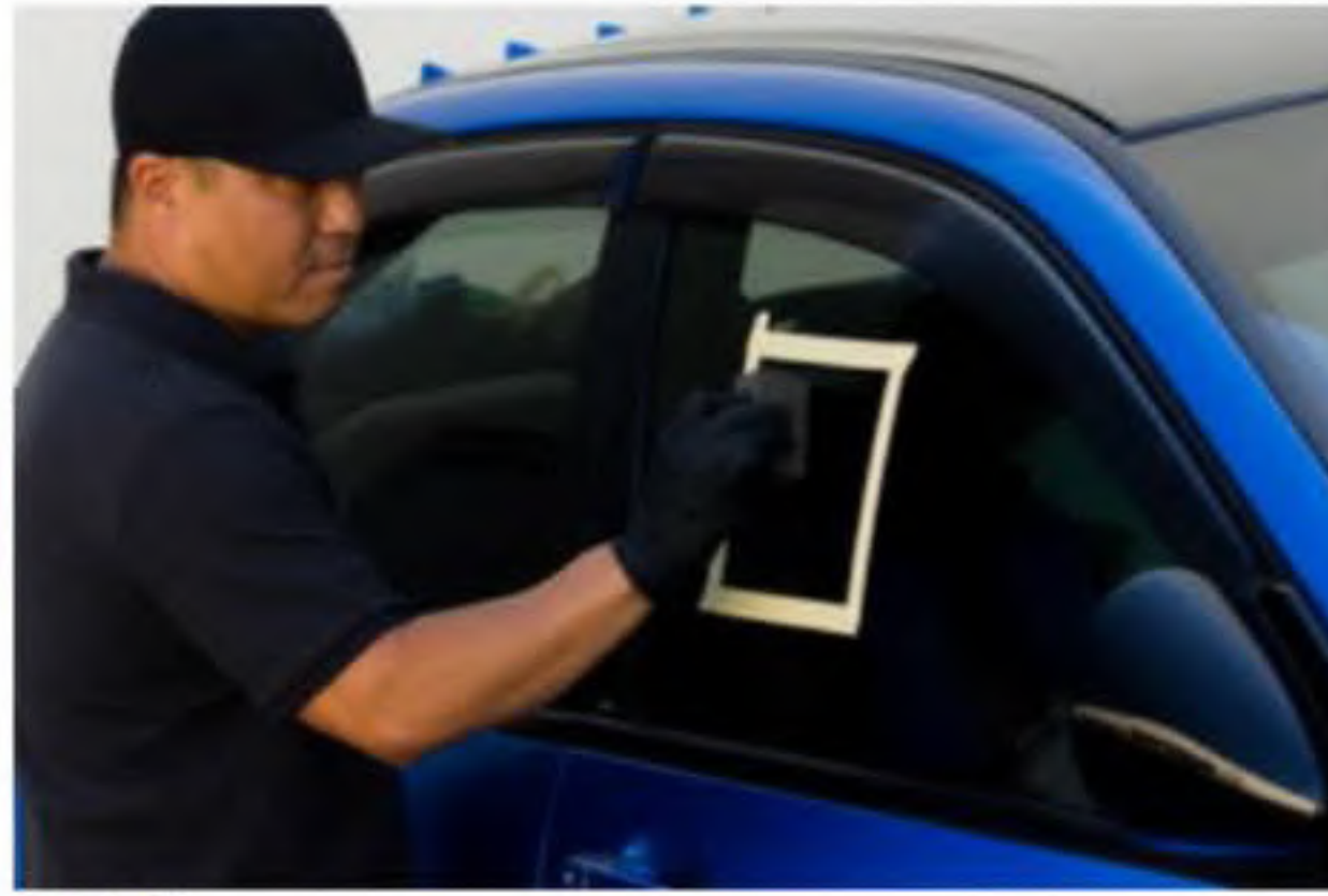
Step 2: Using the rubber polymer side of the included Autoscrub sponge, work the surface back and forth with light to medium pressure. *do not allow Rain Prep to run dry while working with Autoscrub
