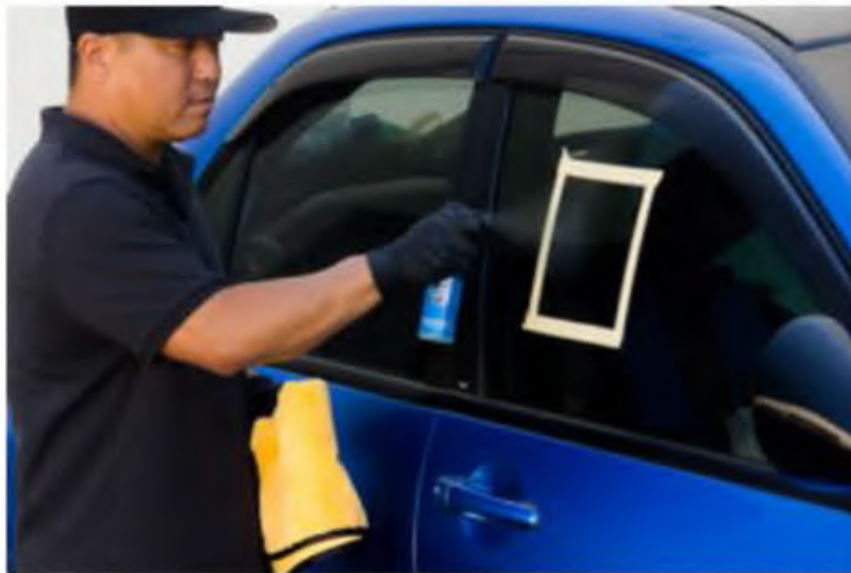
Step 4: Apply Rain glass sealant on previously prepared Rain Prep glass surface
