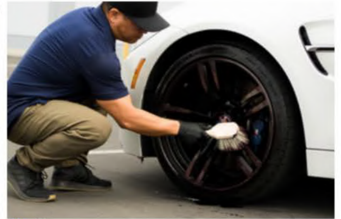
Step 2: Agitate Iron Free with soft wheel brush if necessary for heavily contaminated and neglected wheels
