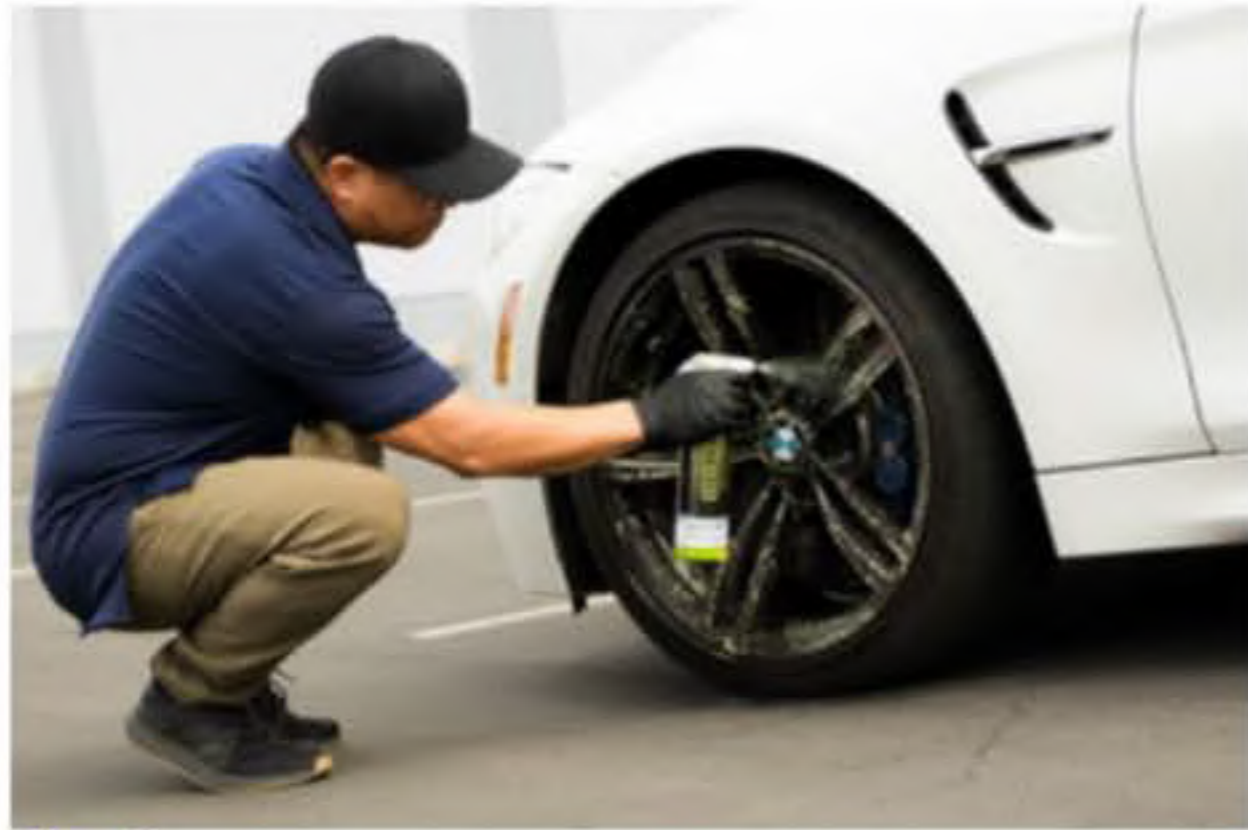
Step 1: Spray a generous amount on wheel, wheel barrel, and brake caliper. *do not apply to hot wheel *use eye protection
