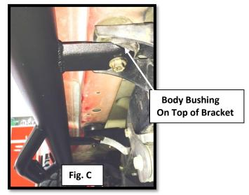
**Step 4:** Next, install the front body bolt and bushing and loosely tighten... **NOTE:** Be sure the round opening in the step bracket fits around the upper body bushing and set s flush with body mount not to pinch the bushing. Fig. D
