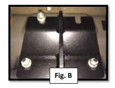
**<u>Step 5</u>**: Staring with the rear bracket, push up towards the pinch weld so the 3" main bar is as high and tight to the body as possible. Tighten all three 8mm flanged nuts.
