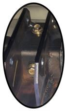
Use supplied M8x30 hex bolts and washers for pinch weld mounts.
