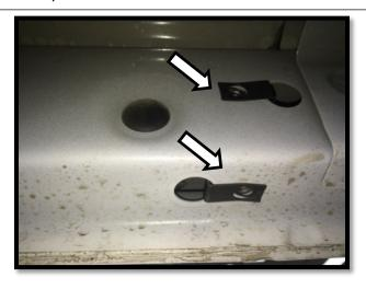
**Step 4:** Next, remove the front and center body bolts and set aside. <u>Do not remove the bushings.</u>
