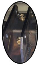
Use supplied M8x30 hex bolts and washers for pinch weld mounts.
