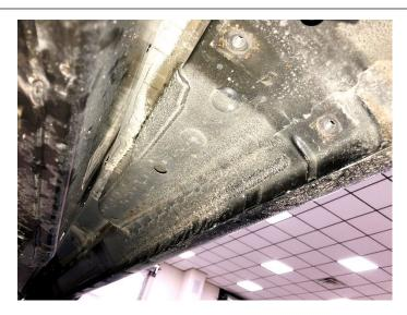
**STEP 3:** Carefully place step into place and loosely fasten using the supplied M10X25mm hardware.
