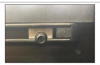
**Step 4.** Next, slide the two remaining bolt and nut assemblies half way through the channel.
