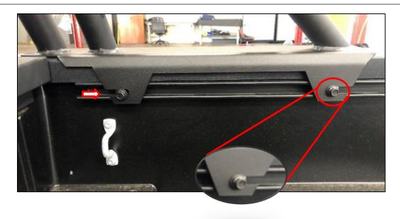
Step 9. Tighten all four mounting positions to 16 ft/lbs (+/- 2lbs).
