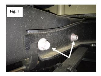
**Step 9:** Remove the 4 OE (both sides) bolts from the frame that attaches the front part of the
