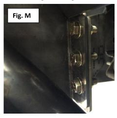
**Step 13:** Align brackets and bumper to desired position and fully tighten hardware. **Note:** *An aftermarket license plate light is recommended.*
