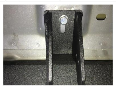
**Step 5.** Next, go ahead, install the two remaining M8x30mm hex bolts in the upper mounts, and leave loose at this time.
