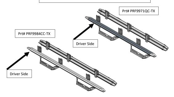
**Step 2** Starting with the Driver side, locate the holes for the upper mounts (x3) and install the supplied (x2) 3/8" clips in each position.
