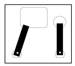
**Step 5:** Align the Nerf Step brackets with the three mounting locations on the underside of the vehicle. Start all six 3/8" x 1" hex bolts with washers and hand tighten.
