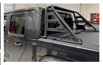
**Step 1**: Attach the Center section to the driver and passenger side assemblies using the supplied 3/8" x 1" carriage bolt (x4) and 3/8" fanged nut (x4) and leave finger tight for now. \*NOTE: Begin with the upper bolt and nut first to have easier access to the lower fasteners. \*
