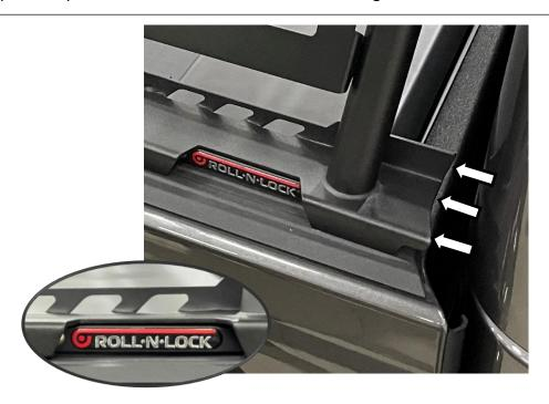
**Step 3:** Slide (x6) threaded channel nuts through rear opening of the T-slotted bed rail and align with the mounting holes in the Sport Bar.
