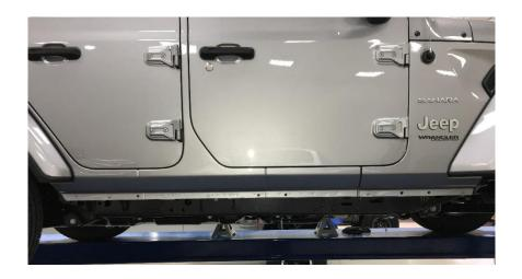
**Step 3.** Starting with driver side step; carefully raise up into position and align the brackets with the factory mounting points with the horizontal part of the bracket on the outside of the pinch weld. **Step 4.** Next, start one of the supplied M8x30mm hex head flanged bolt and washer starting with the center bracket in the factory threaded hole and leave loose.
