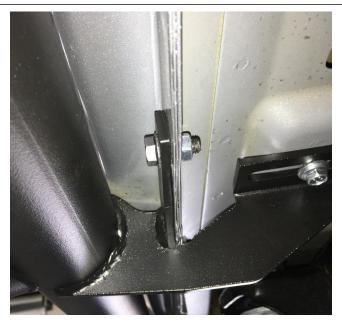
**Step 6.** Continue installing the rest of the hardware in the remaining brackets and leave loose. **Step 7.** Adjust the nerf-step where the main bar is level with the body of the vehicle.
