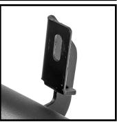
Insert spring loaded U nuts to the body of the truck. There is three per side. The front and rear clips need to be installed facing the rear of the truck.
