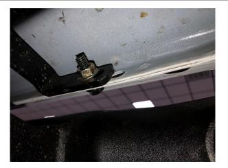
**Step 8:** Begin tightening the lower attachment points starting with the rear bracket working your way up to the front bracket. **( 20ft/lbs )**
