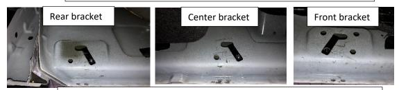
U-clip positioning. *NOTE: Clips will also face forward for passenger side.*
