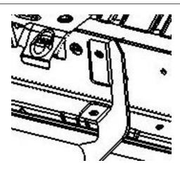
**Step 4** After final adjustment tighten all the lower mount first then the upper mounts.
