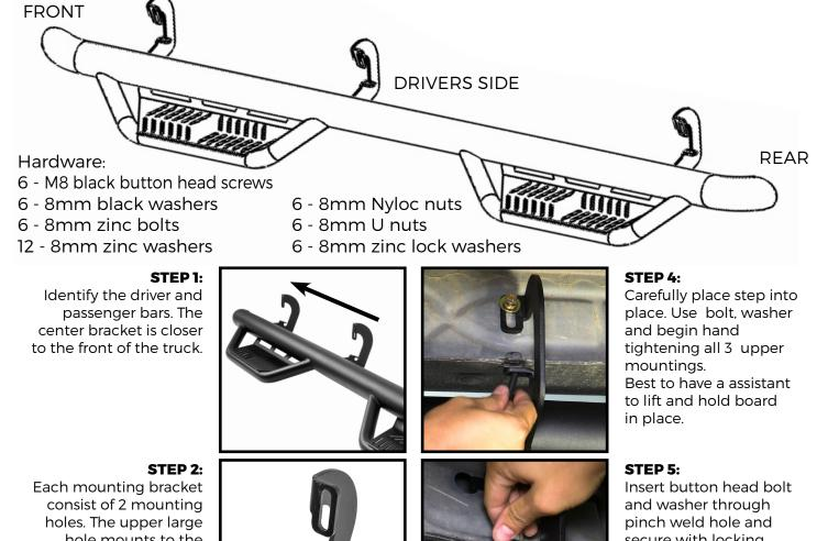
consist of 2 mounting holes. The upper large hole mounts to the body of the truck and the lower smaller hole to the pitch weld.
