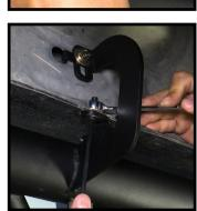
and washer through pinch weld hole and secure with locking nut and washer. With some 1500 models the pinch weld will have a OE nut welded to the truck.
