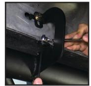
**STEP 6: Avoid using power or air tools.** Tighten pinch weld mounts first then upper bolts. Tighten to 20ft lbs torque to secure the board to the truck. Repeat the same procedure to the other side.
