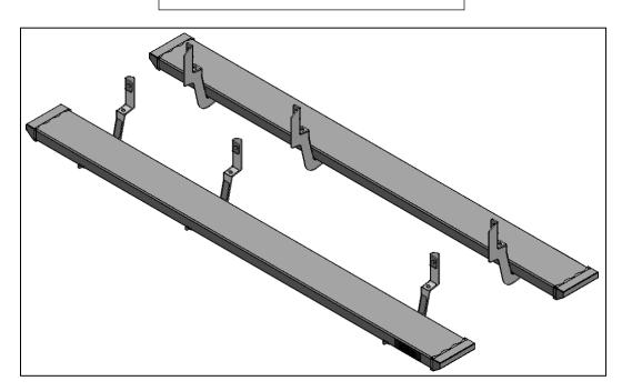
**Step 1:** Beginning with the driver side, remove factory-running bards if equipped and discard. You will see the 8mm threaded mounts in the body. Do the same with passenger side.
