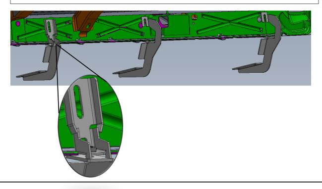
**<u>Step 5:</u>** Set running board along the top of all four brackets and center along the cab.
