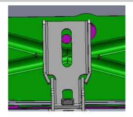
**<u>Step 3</u>**: Using the supplied M8x25mm hex bolts and washers begin hand tightening both upper and lower mounts to the rear two brackets.
