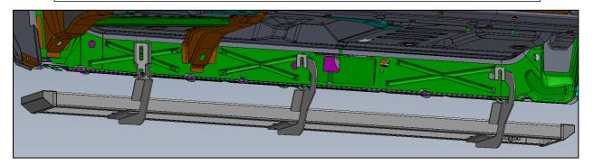
**Step 6:** Insert the supplied threaded brackets (x3) inside the running board lip over the top of each bracket.
