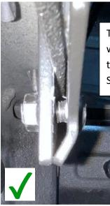
The lip of the bed cap will sandwich between the backing plate and Sport bar.
