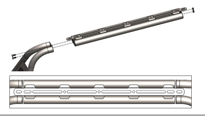
**<u>Step 2</u>**: With additional help, carefully place Sport Bar onto bed rails aligning edge with the plastic cap on both sides.
