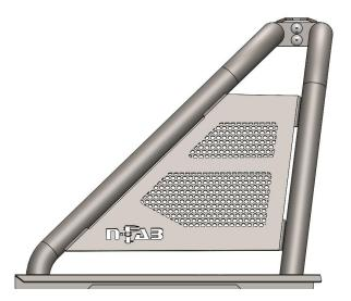
**<u>Step 1</u>**: Attach the Center section to the driver and passenger side assemblies using the supplied 3/8" x 1" carriage bolt (x4) and 3/8" fanged nut (x4) and leave finger tight for now. **\*NOTE: Begin** with the upper bolt and nut first to have easier access to the lower fasteners. **\***
