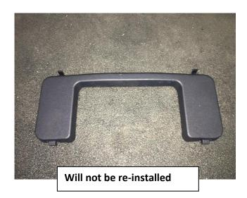
**Step 1:** Remove the plastic tow hook cover by carefully pulling forward to release from bumper. (Both sides)
