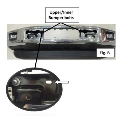
**Step 4:** Using a 3/8" drill bit, drill out the lower mounting hole through the bracket for Driver/Passenger. Secure with supplied 5/16"x1 ½" hex bolt, 5/16" nuts and 5/16" washer.
