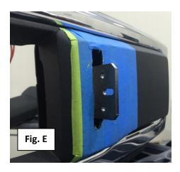
**Step 7:** <u>Install Light bar/Pre-Runner to the bumper brackets</u> using the supplied M6x20mm, M6 flange nuts and M6 washers and leave loose.
