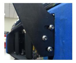
**Step 8:** After Light bar/Pre-runner has been properly adjusted, tighten all hardware. Your install is now complete.
