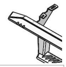
Note: Larger bracket attaches towards the front of the channel
