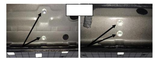
**<u>Step 4</u>**: Position step assembly up to the body of the vehicle and align the brackets up with the factory mounting locations.
