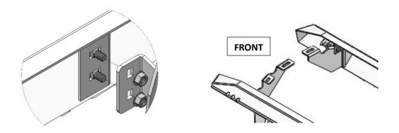
**<u>Step 3:</u>** Remove any factory-equipped running boards, fasteners, and discard.
