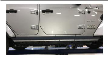
**Step 4:** Carefully raise step assembly into position and align the brackets with the factory mounting points with the horizontal part of the bracket on the outside of the pinch weld.
