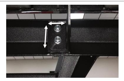
**<u>Step. 8</u>**: After finial positioning, completely tighten all (x6)  $\chi''$ -20 x  $\chi''$  in the pinch weld attachment. **<u>Step. 9</u>**: Next, tighten all (x3) upper body mount positions to 17-20 Ft/lbs. torque. **<u>Step. 10</u>**: Repeat steps 2-9 for passenger side.
