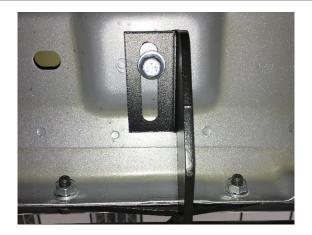
**<u>Step. 6</u>** Next, start all (x6) ¼-20"x 3/4" hex bolts, (x12) M8 flat washers, (x6) 5/16" lock washers and (6) ¼"-20 HC Nut in the pinch weld mounting locations and leave loose for now.
