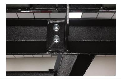
**Step 7:** Adjust the step rail to where you have approximately  $\frac{1}{2}$  gap between the body of the vehicle and the top of the rail.
