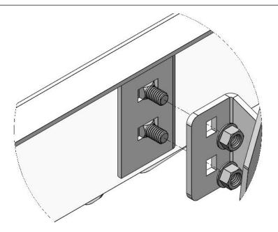
**Step 3:** Starting with the Driver Side. Remove all 8mm flange nuts from the 8mm factory threaded studs to remove the OE running boards.
