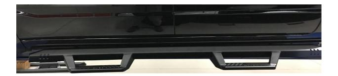
**Step 8:** After finial adjustment, tighten all rocker panel brackets to 30 ft./lbs.
