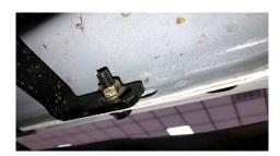
Step 8: Begin tightening the lower attachment points starting with the rear bracket working your way up to the front bracket. (20ft/lbs)
