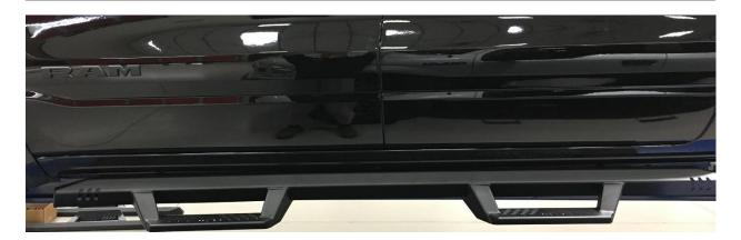
**Step 8:** After finial adjustment, tighten all rocker panel brackets to 30 ft./lbs.
