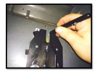
**Step 7:** Remove Nerf Step and set aside. Next, slide the additional 3/8 threaded clip from the upper rectangle hole and align with the "U" shaped mark. Make a mark through the threaded part of the clip.
