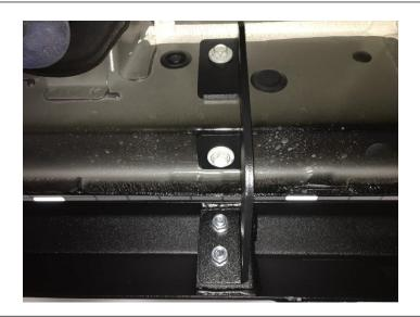
**Step 8:** Repeat steps 2-8 with the passenger side. *NOTE: Periodically check all hardware for tightness to insure longevity and safety of your steps.*
