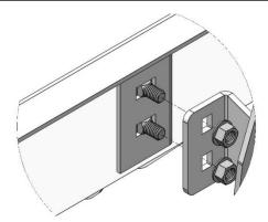
**<u>Step 3</u>**: Remove factory-running bards if equipped and discard. You will see the 8mm threaded mounts in the body.
