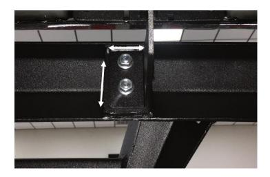
**Step 7:** After finial adjustment, tighten all hardware starting with the three lower bolts and then finish with the upper bolts.
