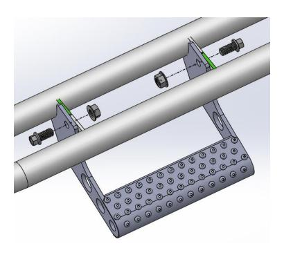
Step 2: Torque bolts to a target torque of 40 ft.-lbs. / 54Nm
