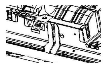
**Step 4** After final adjustment tighten all the lower mount first then the upper mounts.
