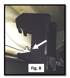
**Step 5:** After final positioning, start at the rear of the vehicle and tighten the lower portion of the bracket to 15-20 ft/lbs of torque. Continue this until all of the lower have been tighten then move to the top bolt and repeat the process.
