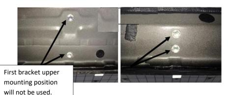
**Step 3:** Position step up to the body of the vehicle and align the brackets up with the factory mounting locations.
