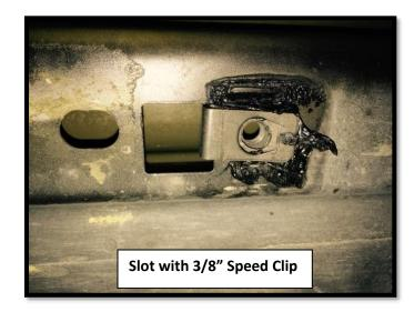
**Step. 3** Carefully raise step rail up to the pinch weld of the body and align brackets up with the factory mounting locations.
