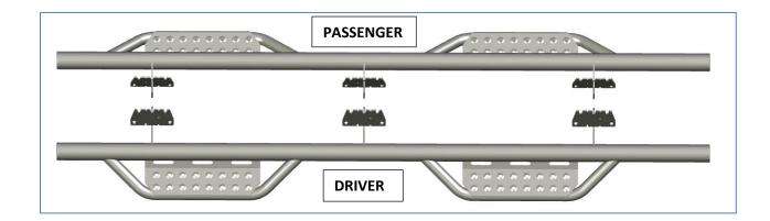
Step 2: Starting with the driver side, remove any steps and old hardware from the vehicle.
