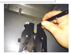
**Step 7:** Remove Nerf Step and set aside. Next, slide the additional 3/8 threaded clip from the upper rectangle hole and align with the "U" shaped mark from step 5. Make a mark through the threaded part of the clip.
