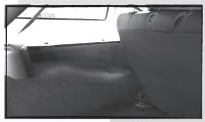
Locate the rooftop mounting bolts as shown (driver side, behind the rear seat above the wheel well). **Note:** Enclosure does not fit convertible version.
