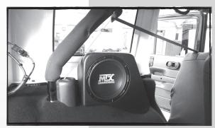
Make all final wire connections (See Page 2), and mount the enclosure into place using the bolts removed from the rooftop mounting location in Step 1.
