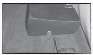
From the driver side, attach the second bracket to the enclosure as shown. Use the same screws from Step 2.
