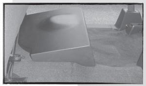
Flip up the driver side rear seat and place the enclosure on the floor as shown above. The enclosure should be inside the seat trim when the seat is in the lowered position.
