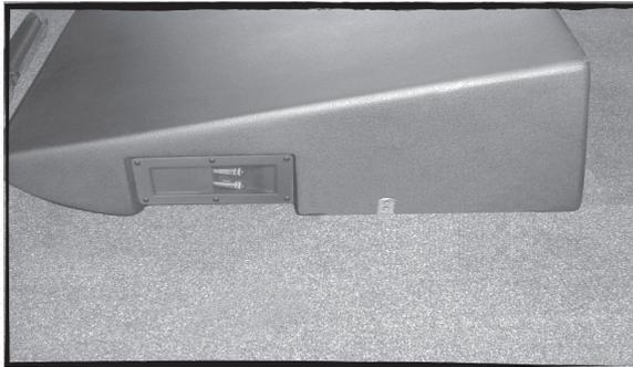
From the passenger side, attach the second bracket to the enclosure as shown. Use the same screws from Step 2.
