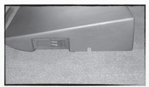
From the passerger side, attach the second bracket to the enclosure as shown. Use the same screws from Step 2.
